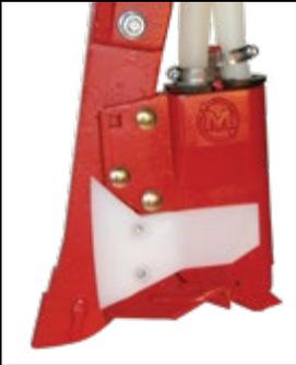
Optional mud guards reduce soil build-up on double-shoot openers. Optional air hose grommets for double-shoot openers prevent straw and debris from falling into the top of the opener ports.
