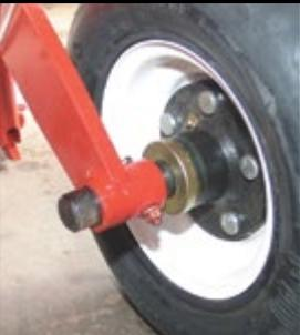
An enclosed shield and seal protects the hub bearings from mud and debris.
