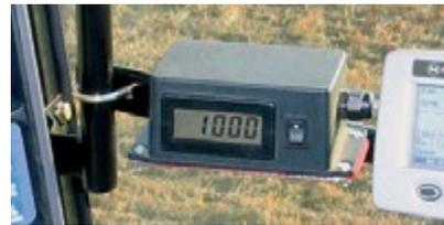
Once set, pressure can be observed from the tractor cab on a convenient digital display.
