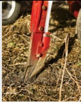
The true one-to-one parallel linkage maintains a constant opener angle relative to the soil and constant opener depth relative to the packer wheel throughout its 17-inch range of travel. The opener can contour up 10 inches and down 7 inches.
