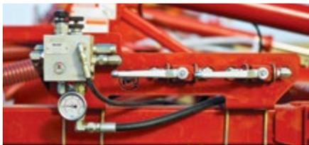
A hydraulic valve manifold providing all operator adjustments is conveniently located on the front bar of the drill.
