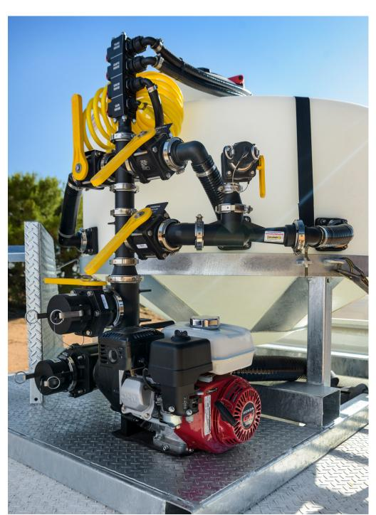
Banjo Venturi Induction system for fast transfer from envirodrums and shuttles
